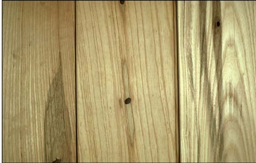
Figure 30: Ash Lumber, with Ash Borer Damage (Photo: James Solomon, USDA Forest Service)
