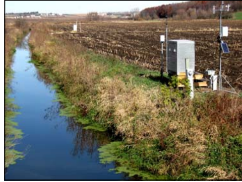
Stream Monitoring Site: This USGS monitoring site records stream flows and collects water quality samples to determine suspended sediment, phosphorus, and nitrogen concentrations during storm runoff events.
