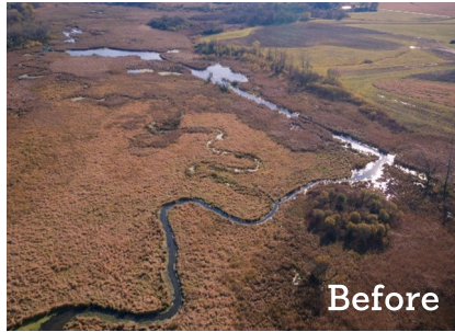
Dorn Creek had left its original channel and was flowing through a nearby agricultural ditch. Part of this project included restoring the stream to its original, meandering river channel.
