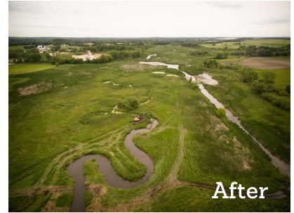
Dorn Creek had left its original channel and was flowing through a nearby agricultural ditch. Part of this project included restoring the stream to its original, meandering river channel.
